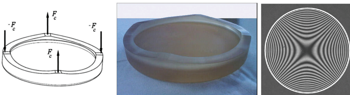
Figure 30 Left and center: Elasticity design in CTD class, i.e., t/t_0 = \text{constant} , of a 40-cm mirror in Zerodur vitrocera bent by four forces during stress figuring. Its contour realizes a built-in boundary to a ring whose axial thickness t_r(\theta) shows four azimuth thickness narrowings , t_{R-\text{Max}}/t_{R-\text{Min}} = 1.16 , to ensure an accurate modulation in \cos 2\theta . Right: He-Ne interferogram with respect to a mean curvature sphere of one of the three Astm3 -correcting mirrors made for SPHERE. This instrument is a next-generation planet finder of the ESO-VLT (LOOM, Thales SESO Corp.).
