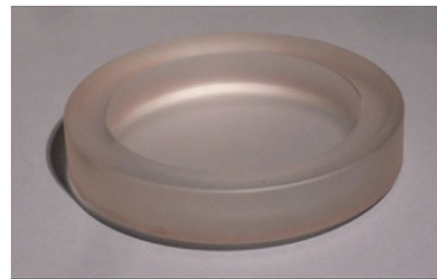
Figure 37 Left: Convex vase form mirrors parabolized by stress figuring. Right: View of a fused-silica ULE mirror for the GI2T (LOOM).
